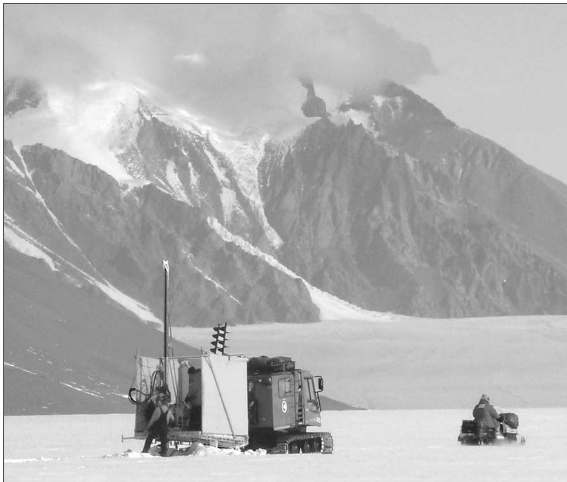
Working on eight-foot thick sea ice, researchers use a giant air gun to probe sediments beneath the ocean floor.
